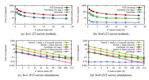
Figure 7: Varying the number of reduce tasks using S=0 and S=1 workloads (log-scale).
