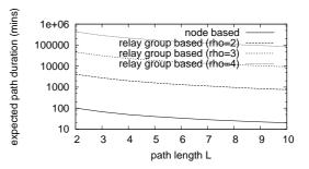
Figure 10: Comparing expected durations of node-based paths and "relay group"-based paths with intermittent failures. (Note:  $\rho$  is shown as "rho"; y-axis is log-scaled.)
